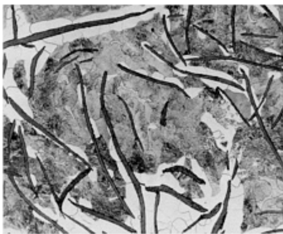
Fig. 4 Microstructure of a gray cast iron with a ferrite-pearlite matrix. 4% picral etch. 320×. Courtesy of A.O. Benscoter, Lehigh University
