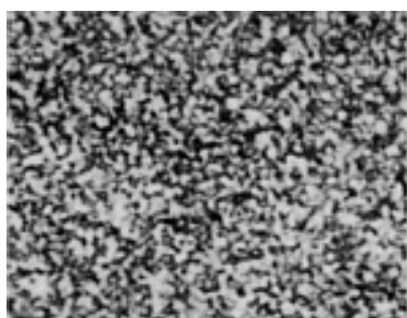
Fig. 18 Photomicrograph of Zn-22Al alloy (eutectoid composition) showing superplastic, fine-grained structure obtained by annealing at 350 °C (660 °F) and water quenching. 2500×
