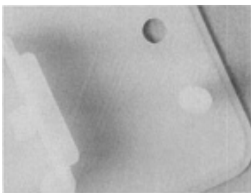
Fig. 10 Porous texture of parts made using FDM caused by adjacent lines of polymer that do not fuse together perfectly
