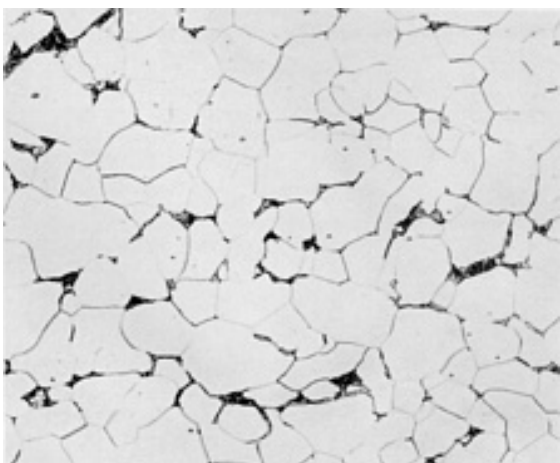
Fig. 10 Photomicrograph of pearlite (dark constituent) in a low-carbon steel sheet. 2% nital + 4% picral etch. 1000×
