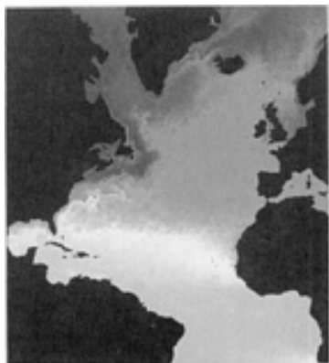
Fig. 2 Ocean surface temperatures from a recent CFD simulation of the North Atlantic Ocean. Source: Ref 8
