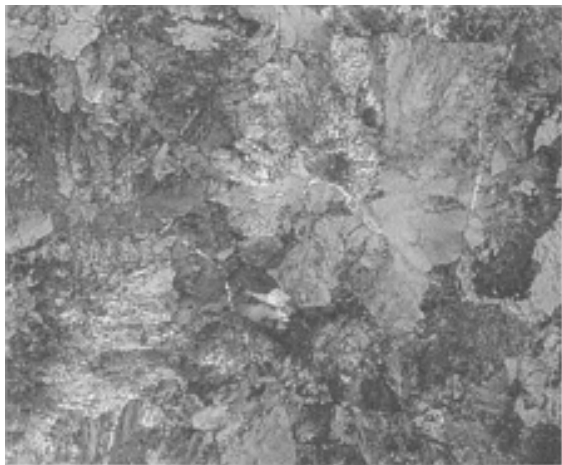
Fig. 3 Microstructure of a typical fully pearlitic rail steel showing the characteristic fine pearlite interlamellar spacing. 2% nital + 4% picral etch. 500×
