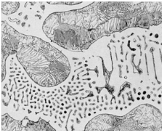
Fig. 49 Microstructure of the eutectic constituent ledeburite in a typical white cast iron. 4% picral etch. 500 \times . Courtesy of A.O. Benscoter, Lehigh University
