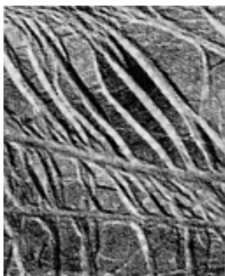
Fig. 36 Stretcher strains (Lüder's bands) in rimmed 1008 steel
